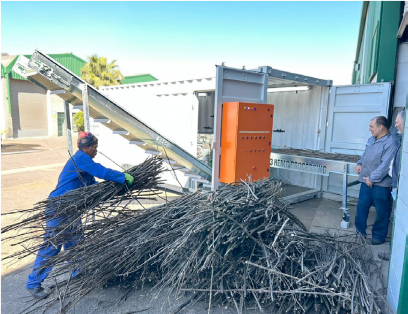
Figure 10. Landrace Stalks from Mpondoland Tested for Mobile Decortication
