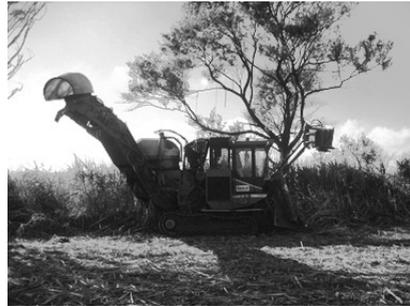
**Photo 6:** Machine used for mechanised cutting of unburnt cane. Region of Andradina, Sao Paulo. Xavier, C. V. May 2011.
