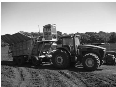
*Photo 1: Equipment used in mechanised sugar cane planting. Supplier farm of cane for Gaza plant (Cosan), in the municipality of Andradina (Sao Paulo state). Xavier, C.V. May 2011.*
